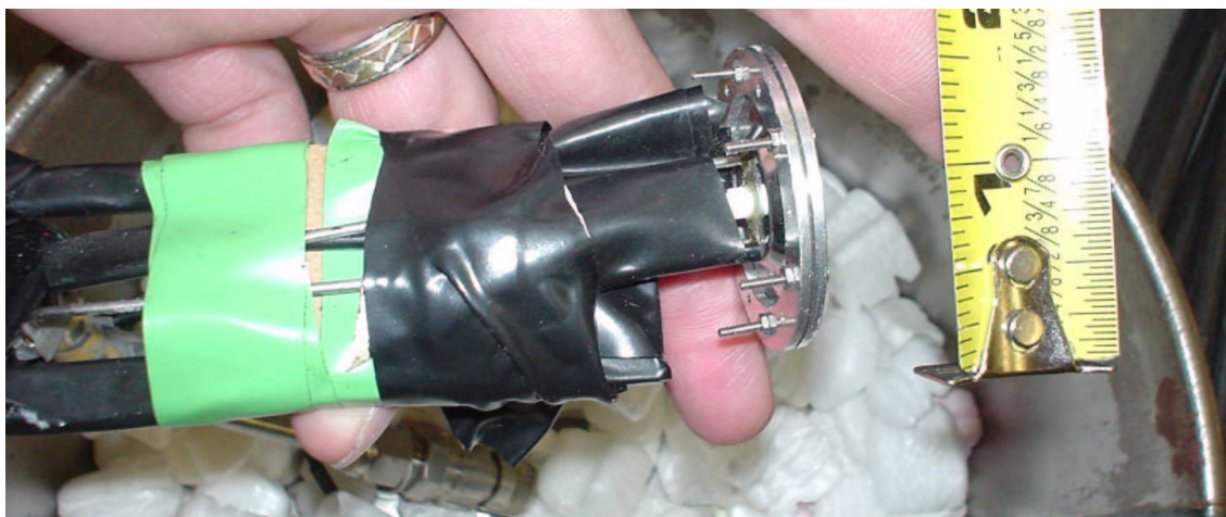
Figure 1: ^{252}\text{Cf} chamber with methane and electrical lines.
